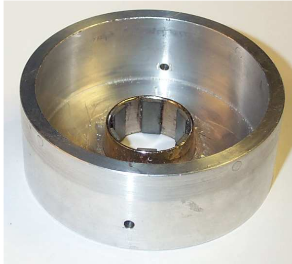
Figure 5.13: The brushless DC motor's rotor and permanent magnets mounted on the 3Dwheel's aluminium liner.
