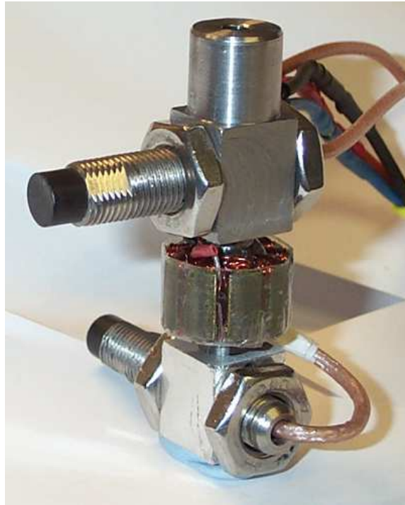
Figure 5.12: The brushless DC motor's stator mounted between the two translation eddy current sensors.
