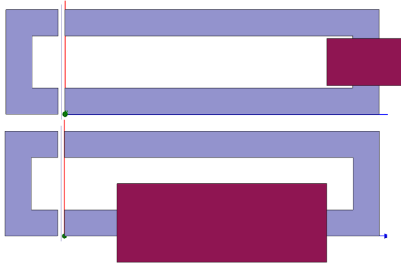
Figure 4.12: A finite element simulation of identical electromagnets with their coils mounted in different locations. The top electromagnet has a coil on its back edge and the bottom magnet has the coil on its bottom edge.
